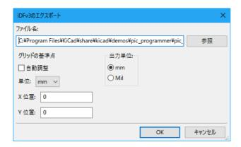
**Grid reference point:** Choose where the exported model's reference point should be. If the **Adjust automatically** option is selected, KiCad will set the reference point to the centroid of the PCB. Otherwise, the reference point is set relative to the display origin.
