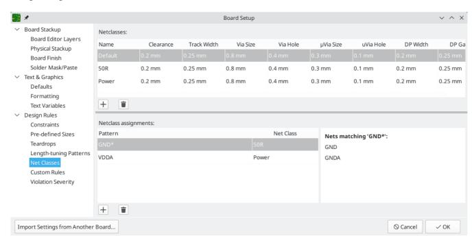
The upper portion of the Net Classes section contains a table showing the net classes in the design and the design rules that apply to each net class. Every class has values for copper clearance, track width, via sizes, and differential pair sizes. These values will be used when creating tracks and vias unless a more specific rule overrides them (see Custom Rules below).
