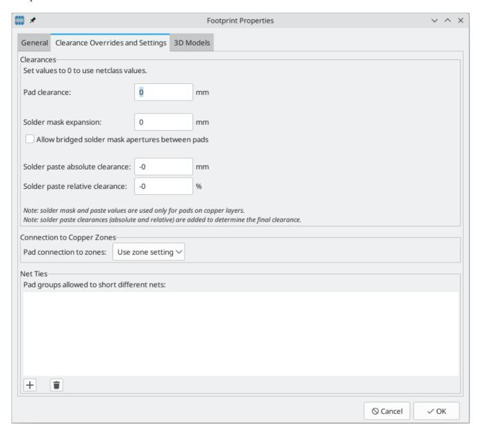
**Pad clearance** controls the minimum clearance between the footprint's pads and any copper shape (tracks, vias, pads, zones) on a different net. This value is normally set to 0 which will cause the pad clearance to be inherited from the board's design rules and netclass rules. This value can be overridden for individual pads by setting the pad's clearance to a nonzero value.
